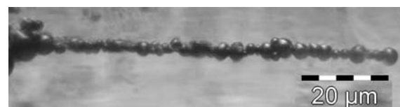
Fig. 2 A chain of the structured composite viewed by optical microscopy at low volume fraction ( \Phi = 3\% ) inside a transparent elastomer
